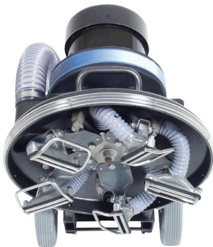
Soiled solution is then extracted from the carpet by five stainless steel cleaning heads and drawn through the aluminum exhaust manifold to your cleaning system's recovery tank.
