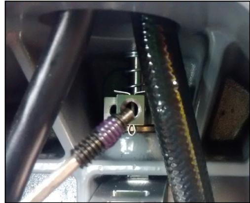
**Figure 9-5. Reinstall dog point set screw**
